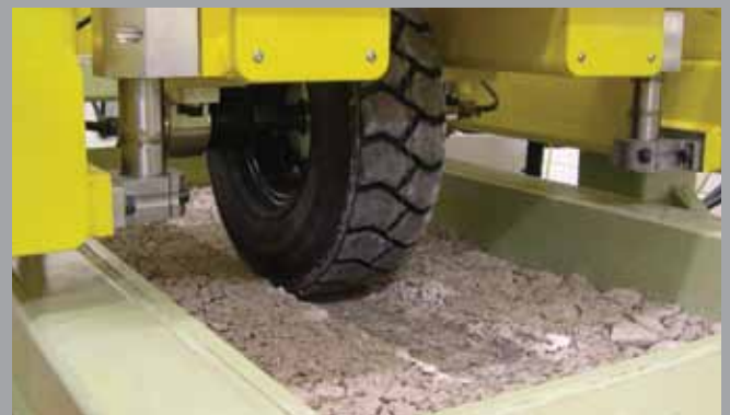
2007 Tensar Technology Centre – In-house trafficking facility enables geogrids, fills and subgrades to be investigated
