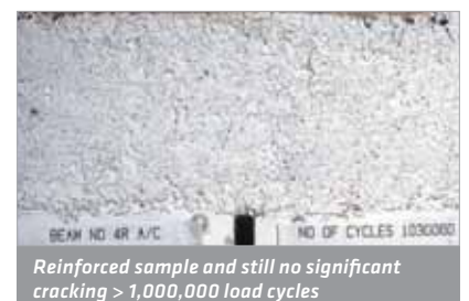
Inclusion of Tensar AR inhibits the development of reflective cracking.
