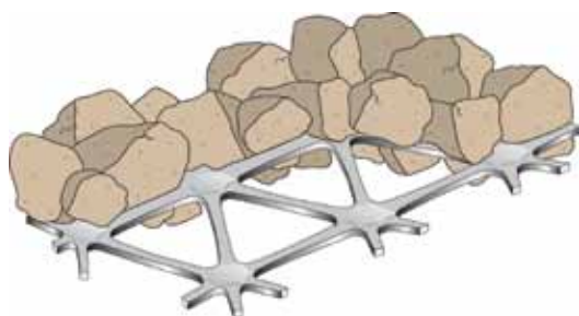
Aggregate particles interlock with the TriAx geogrid and are confined within the apertures forming a mechanically stabilised layer with increased load bearing capacity.
